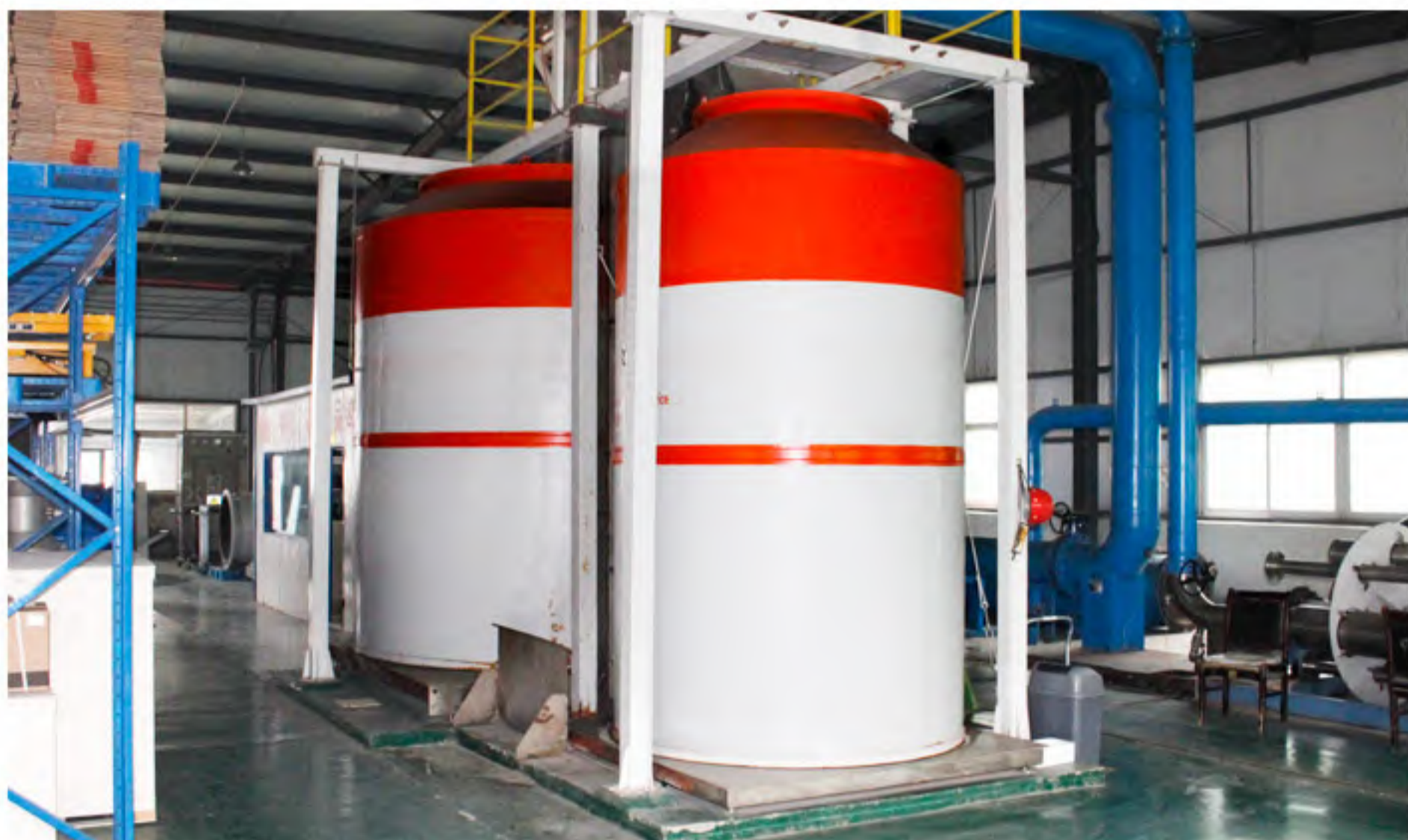
DN350-DN700 & DN65-DN300 0.1 % Weighing and volumetric device to ensure accurate calibration
