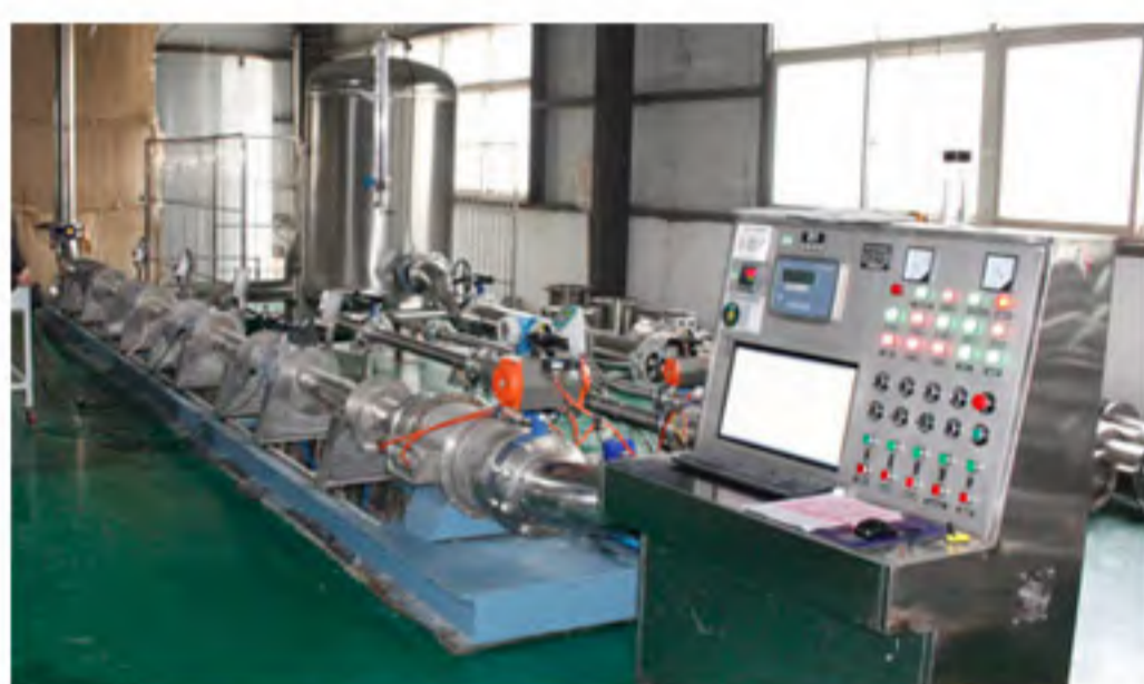
DN65-DN300 Gravimetric & Standard Meter Liquid Flow Meter Calibration Device
