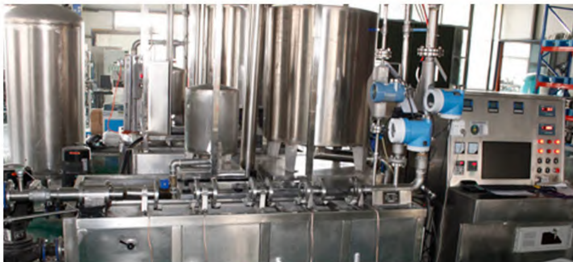
Coriolis Mass Flowmeter Standard Meter DN15-50 Gravimetric & Standard Meter Liquid Flow Meter Calibration Device
